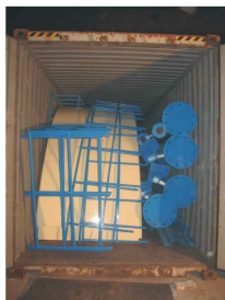
sectional cement silo in container
