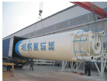
50 tons cement silo in loading
